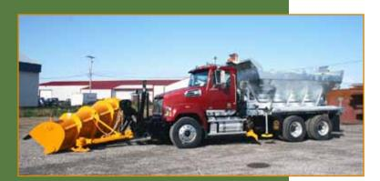
**9** n the past, the Modular Road Salt Spreaders have always been painted, which resulted in a very short service life, high maintenance costs to continuously combat corrosion, and very unpleasant aesthetics, even after only one year of service. This product is an example of how larger galvanizing baths are creating important new markets.
