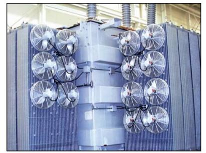
Menk USA decided to hot-dip galvanize the radiators and fan guards because of the coating's durability and corrosion resistance. However, the radiators are very thin and can warp easily, so they require some special handling to ensure they meet the high standards of the transformer industry. By electing to galvanize the cooling radiators, Menk USA delivers a dependable product to its customers that will avoid critical shutdowns and a coating that will remain maintenance-free for many years.
