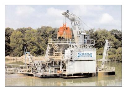
With the objective of designing and building a dredge superior to the competition in performance, uptime percentage, and long-term durability, Supreme Manufacturing had an experience base that suggested there was only one corrosion protection system that would qualify — hot-dip galvanizing.
