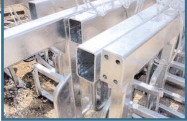
the last 13 years—to use hot-dip galvanized head gates, milking stalls, and tubular rails to support its 6,000-cow dairy operation.
