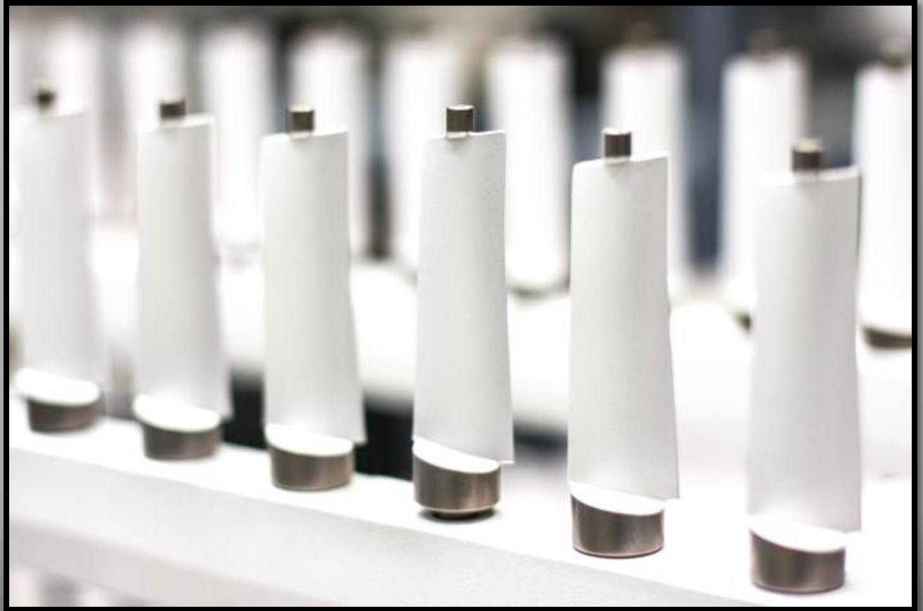
Gas turbine compressor blade, power generation Compressor blades in tooling rack
