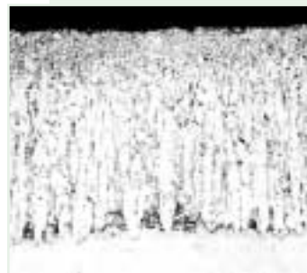
A photomicrograph of a galvanized coating on high silicon content steel.
