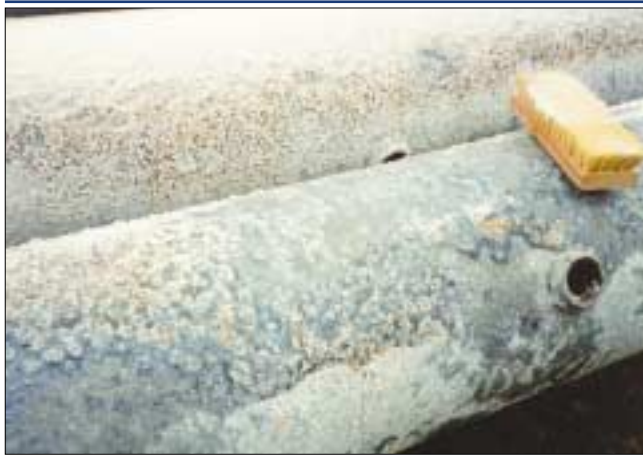
Most parts with a medium layer of wet storage stain, Figures 6 and 7, can be cleaned and then put into service.
