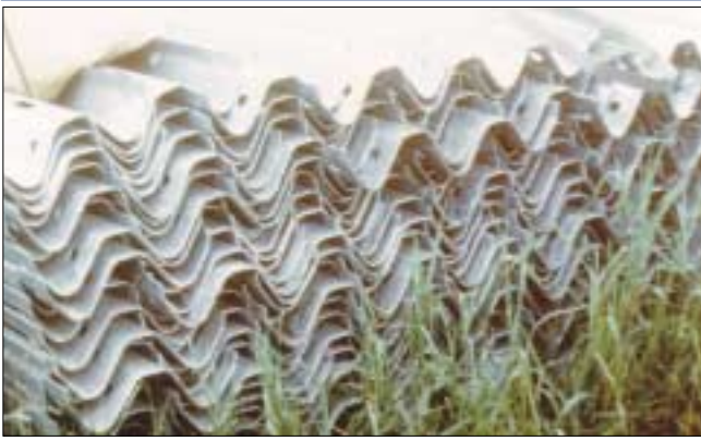
Figure 3 shows improperly stored galvanized guardrail. Storing galvanized steel in vegetation with no spacers between the products creates a highly conducive environment for wet storage stain to take place. By contrast, the items on this truck, Figure 4, are ideally stacked for transportation.
