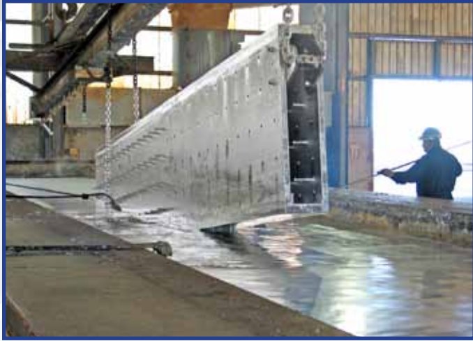
Withdrawal of a steel article from the zinc bath.
