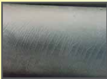
FIGURE 30: STRIATIONS (ACCEPTABLE) FIGURE 31: FISH BONING
