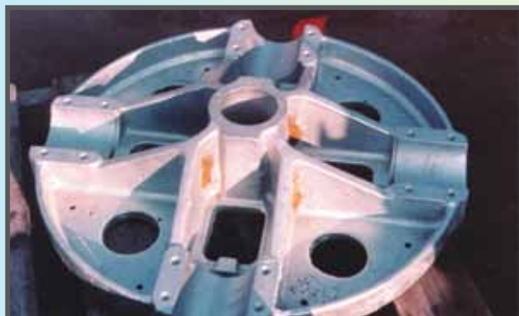
FIGURE 29: SAND EMBEDDED IN CASTING (REJECTABLE)
