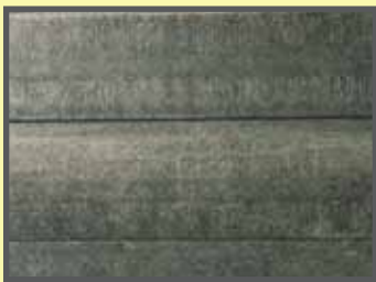
FIGURE 30: STRIATIONS (ACCEPTABLE) FIGURE 31: FISH BONING
