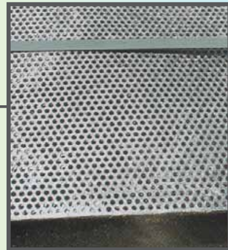
FIGURE 15A: CLOGGED HOLES (ACCEPTABLE)
