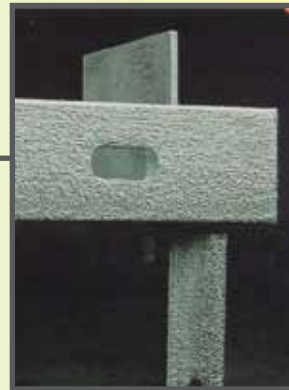
FIGURE 26: ROUGH SURFACE CONDITION/ STEEL SURFACE CONDITION (ACCEPTABLE)
