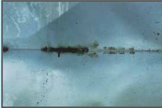
FIGURE 37: ZINC SKIMMINGS (ACCEPTABLE)
