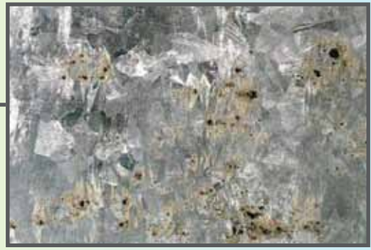
FIGURE 20: EXCESS ALUMINUM IN GALVANIZING BATH (REJECTABLE)
