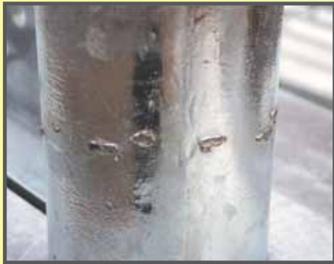
FIGURE 14: CHAIN AND WIRE MARKS (ACCEPTABLE UNLESS BARE STEEL IS EXPOSED)
