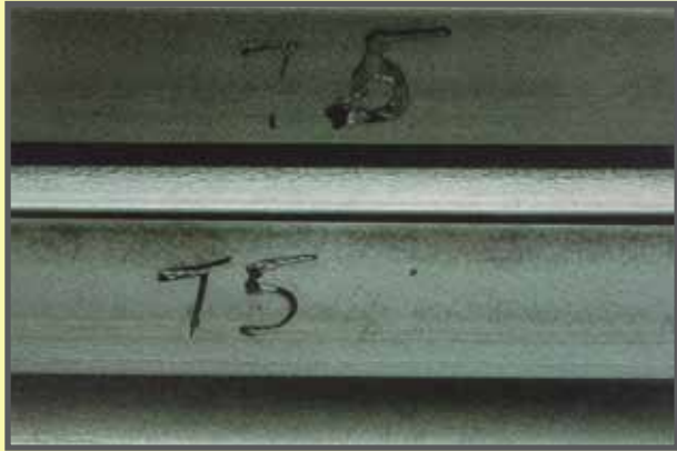
FIGURE 32: SURFACE CONTAMINANT (REJECTABLE)
