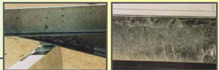
FIGURE 19: DROSS INCLUSIONS (ACCEPTABLE UNLESS LARGE, AND IF REMOVED, A BARE SPOT IS EXPOSED)
