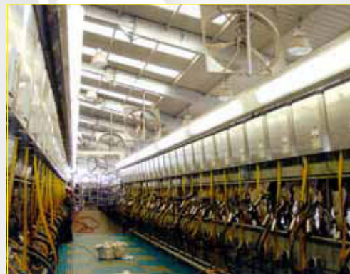
Galvanized steel will protect this milking facility from the corrosive elements of the dairy industry.
