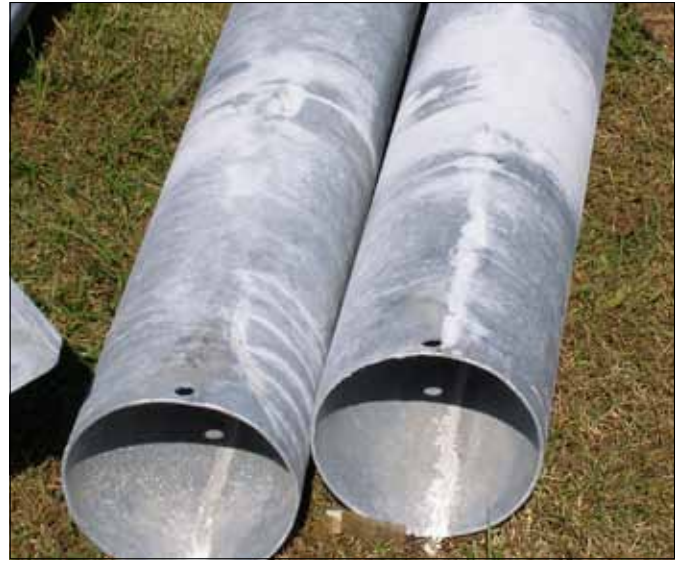
Pipes suffering from wet storage stain.
