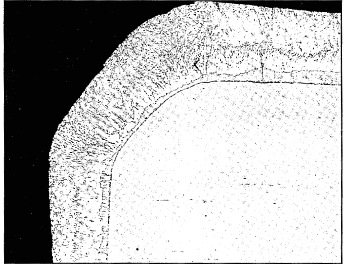
Edge thickness of hot-dip galvanized steel
