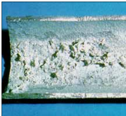
When flux inclusions, above, are removed, the bare steel becomes exposed.
