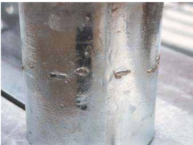
Figure 1: Chain marks on a hot-dip galvanized product.
