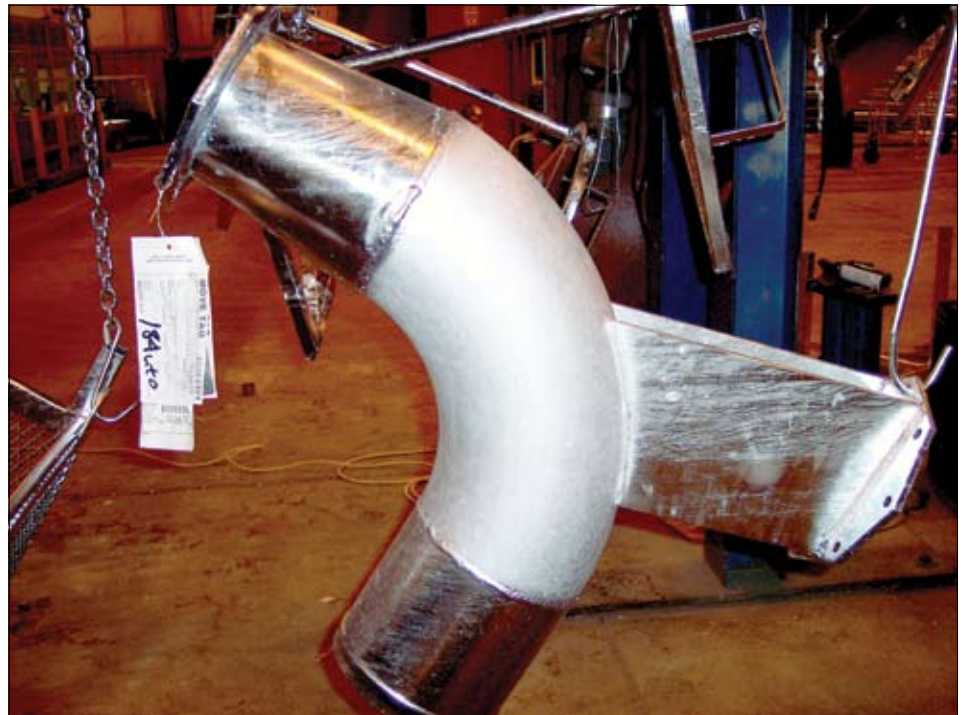
Variations in steel chemistry, surface preparation, kettle chemistry, and steel exposure conditions can cause a difference in coating appearance.
